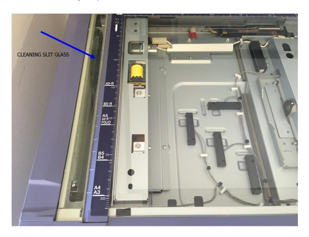
**Step 4** - Use a bit of Steel Wool or Metholatyed Spirits to remove the dirt from the Slit Glass
